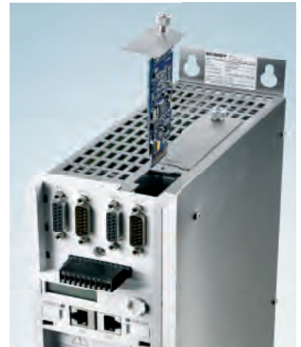
With the AX58xx TwinSAFE drive option card, the AX5000 servo drive is easily converted into a safe drive solution that offers the user numerous safety functions.
