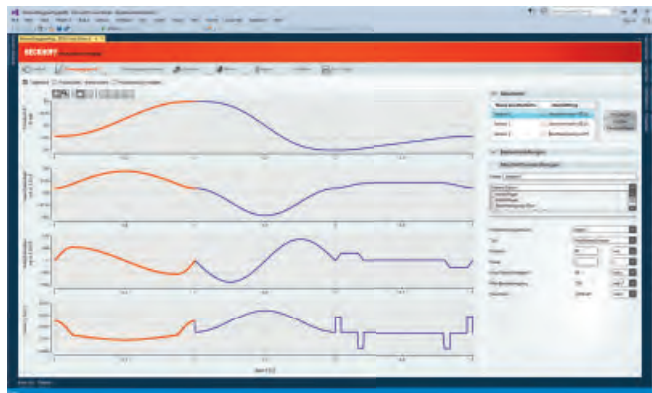
The Motion Designer enables the direct observation of the curves of position, speed, torque and acceleration over time for each axis.
