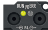
IP-Link interface on the Extension Box for communication with the fieldbus coupler
